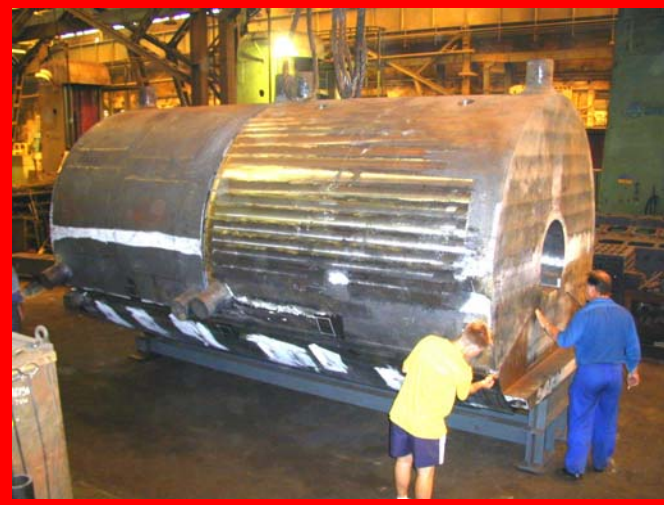
100 tonnes iron shielding pieces being cast in the Czech republic.
